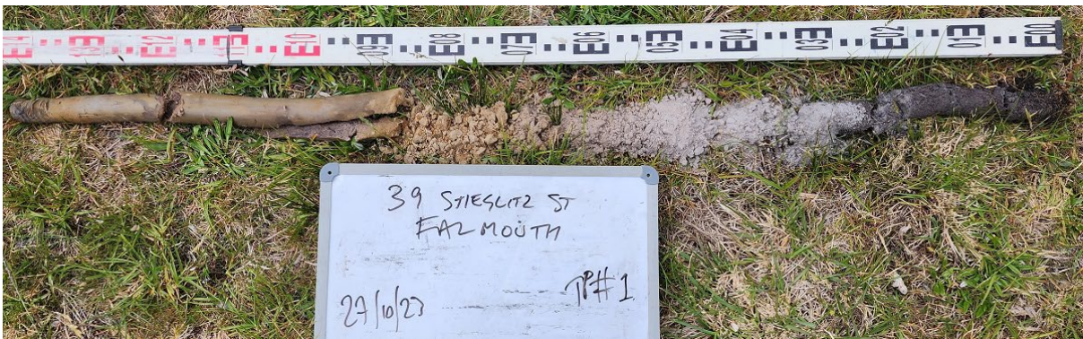
(above) Soil cores to 1400mm from land application area.
