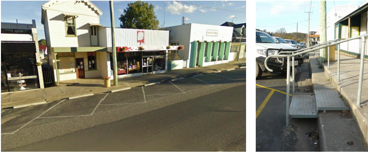
Figures 5 and 6: Kerbing Too High (Photo: Bitzios Consulting and TCG Planning)
