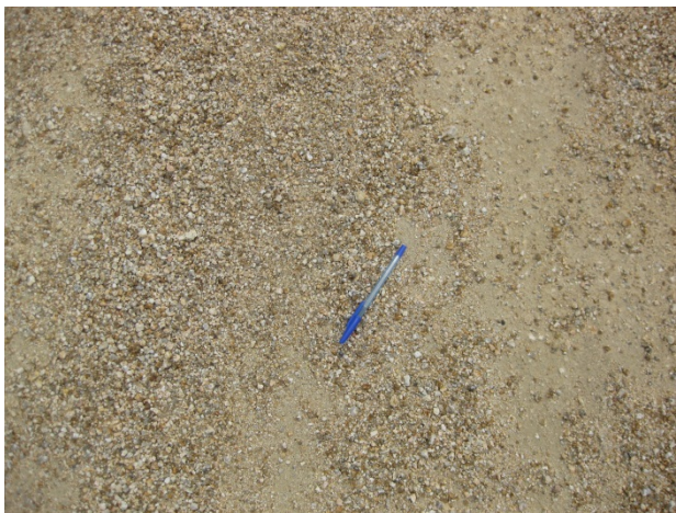
Photo 1 – Typical Runway unbound granular wearing course
