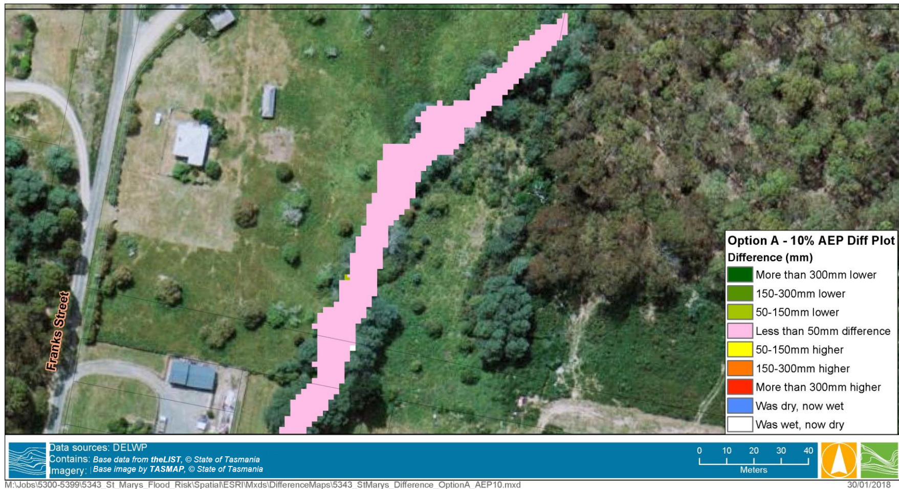
FIGURE 4-4 OPTION A – 10% AEP DESIGN EVENT FLOOD EXTENT ALONG NEWMANS CREEK
