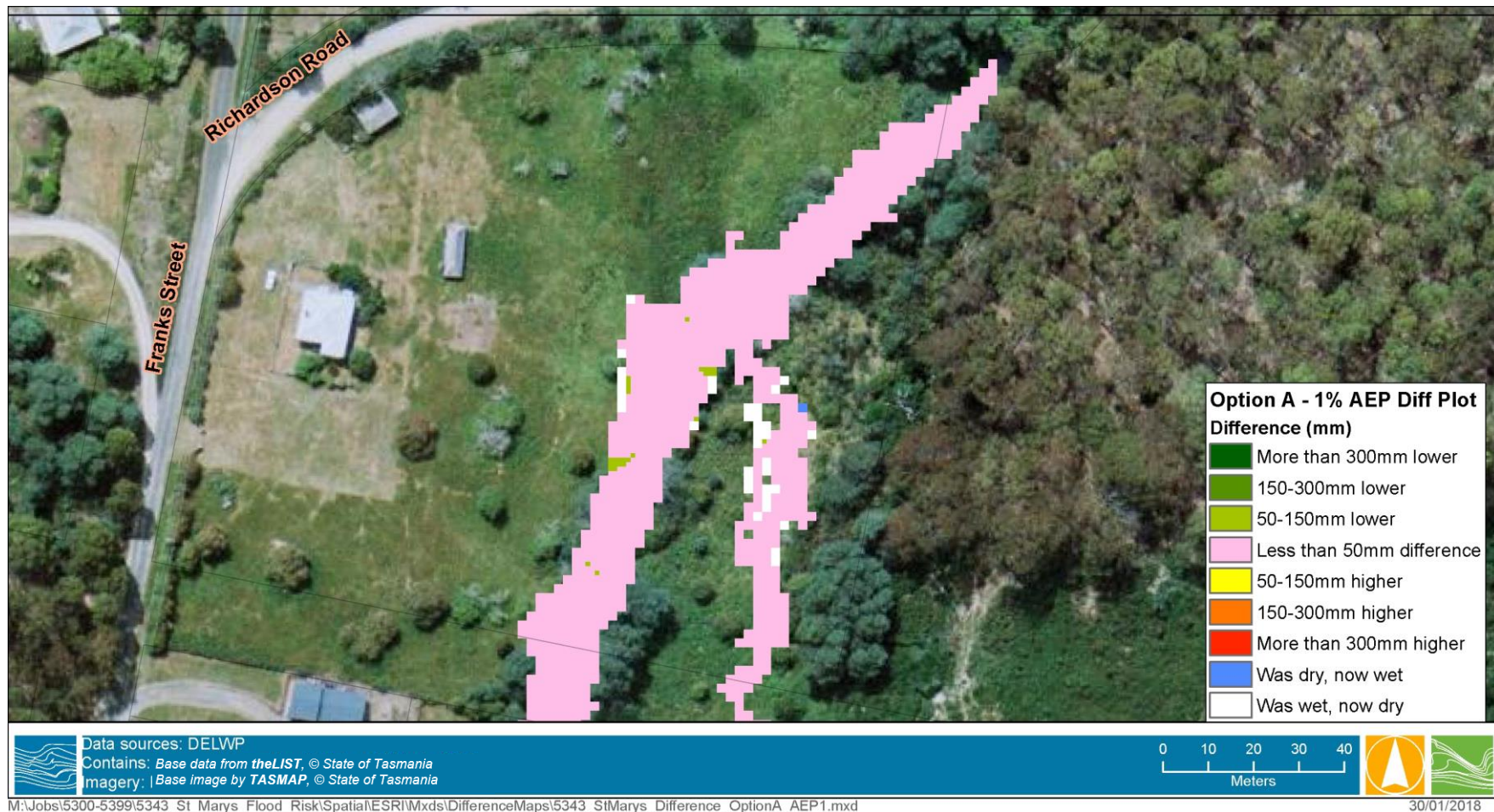
FIGURE 4-5 OPTION A – 1% AEP DESIGN EVENT FLOOD EXTENT ALONG NEWMANS CREEK
