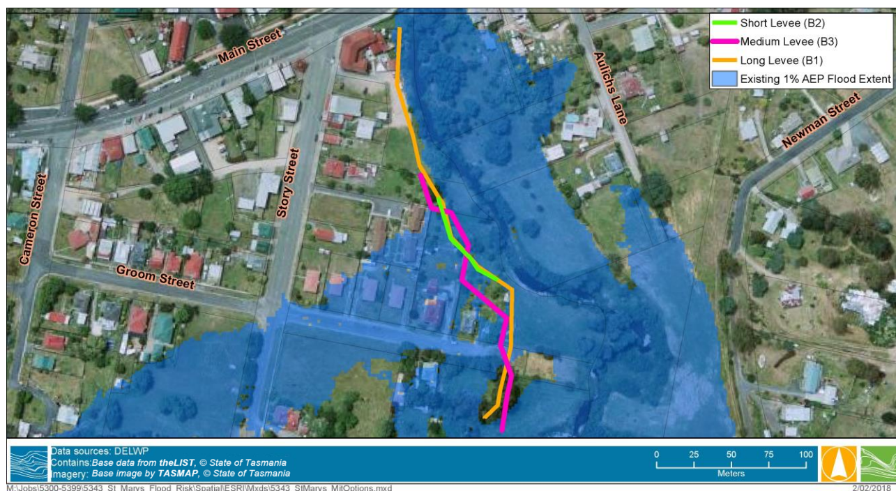
FIGURE 4-6 OPTION B LEVEE ALIGNMENTS
