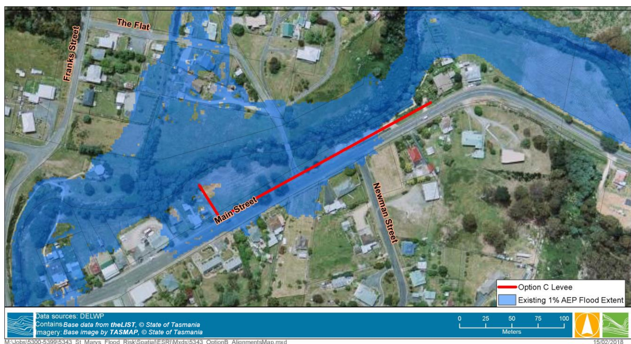
FIGURE 4-13 OPTION C LEVEE ALIGNMENT
