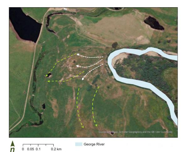
**Figure 6.** The breakout point under scenario 3. White dashed lines show approximate direction water and sediment will move and green dashed lines show the two dominant directions floodwaters may travel, which determines whether alignment 3A or 3B is realised (see Figure 7).
