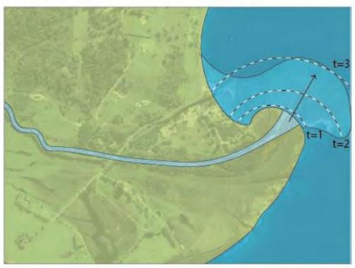
**Figure 1.** The progression of a deltaic lobe at the mouth of the Goerge River and its impact on channel slope. Figure from Water Technology, 2022.
