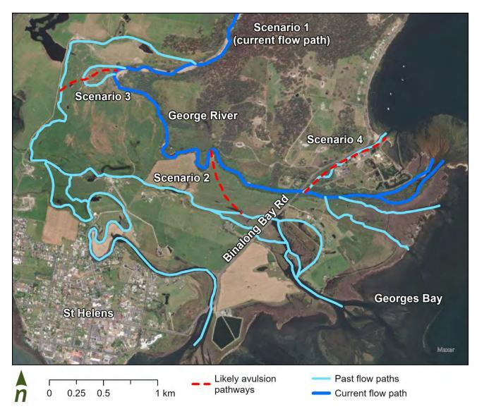
**Figure 3.** Overview of the four avulsion scenarios. Red dashed lines are liekly alignments of newly scoured channel on the floodplain and light blue lines are channels that may be re-occupied by the George River following avulsion.
