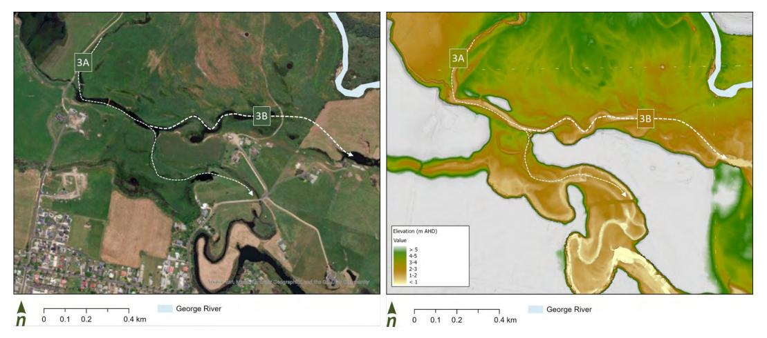
Figure 7. The alignments of two abandoned channel that may be re-occupied by the George River under scenarios 3A and 3B. The George River is likely to re-occupy one (but not both) of these channels under scenario 3.
