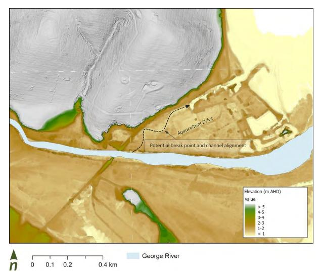
**Figure 8.** The potential alignment of a newly scoured channel under scenario 4 (grey dashed line), adjacent Aquaculture Drive.
