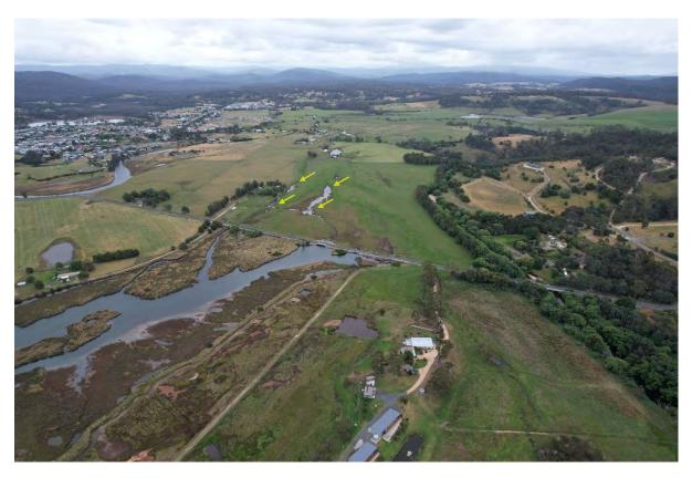
**Figure 4.** Aewrial view of the salt marsh at the edge of Georges Bay which is separated from the George River floodplain by Binalong Bay Road. Yellow arrows indicate scour channel shown in Figure 5.
