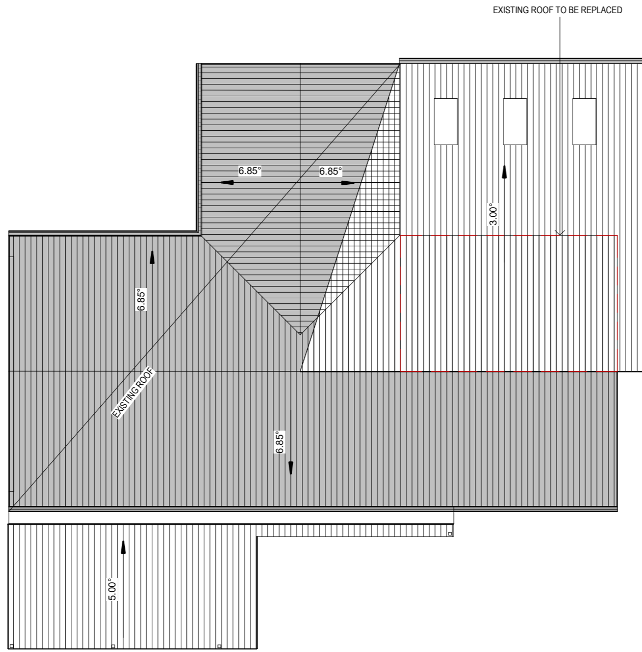
RENOVATION & SUNROOM ROOF PLAN SCALE 1 : 100
