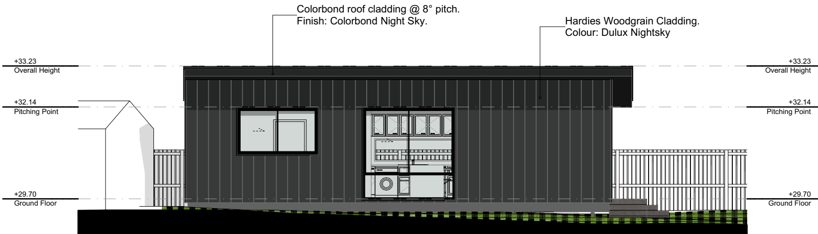
E-03 East Elevation #LayID Scale 1:100
