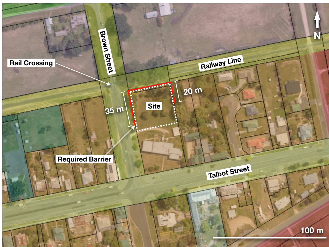
FIGURE 4.1: REQUIRED BARRIER LOCATION
